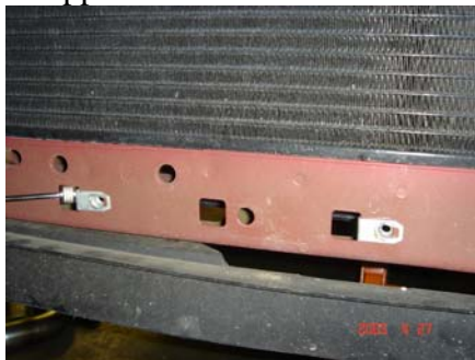
81. Install intercooler with supplied metric bolts and washers as seen
