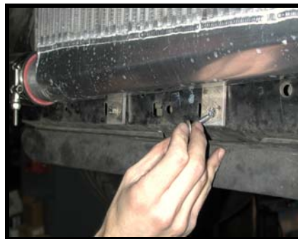
82. Install intercooler support strap to hood latch and intercooler. Hang strap from hood latch and secure with supplied 5/16" hardware.
